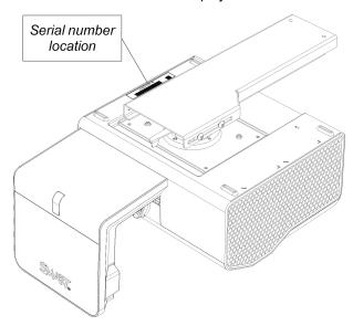
The ECP serial number is located on the bottom of the ECP.
